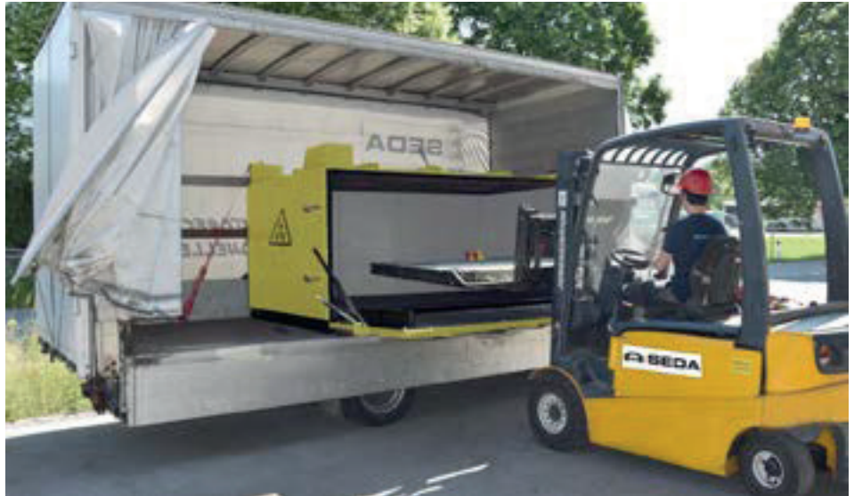
Loading of the HV Bat-Box with Li-ion battery on the truck
