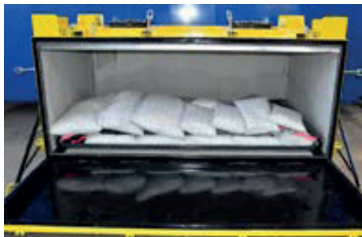
HV Bat-Box when loaded with Li-ion battery and fiberglass pad for filling
