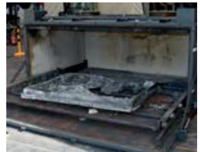
HV Bat-Box with burnt out Li-ion battery
