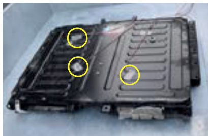
Temperature monitoring with 4 sensors in each box
