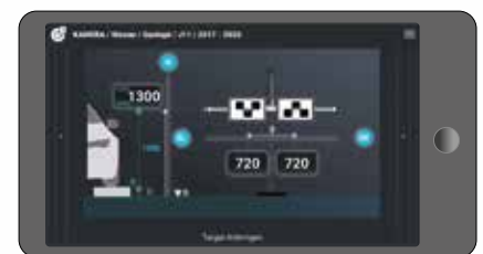
Q.mApp software: Guides the user through the entire ADAS calibration, including live data and documentation
